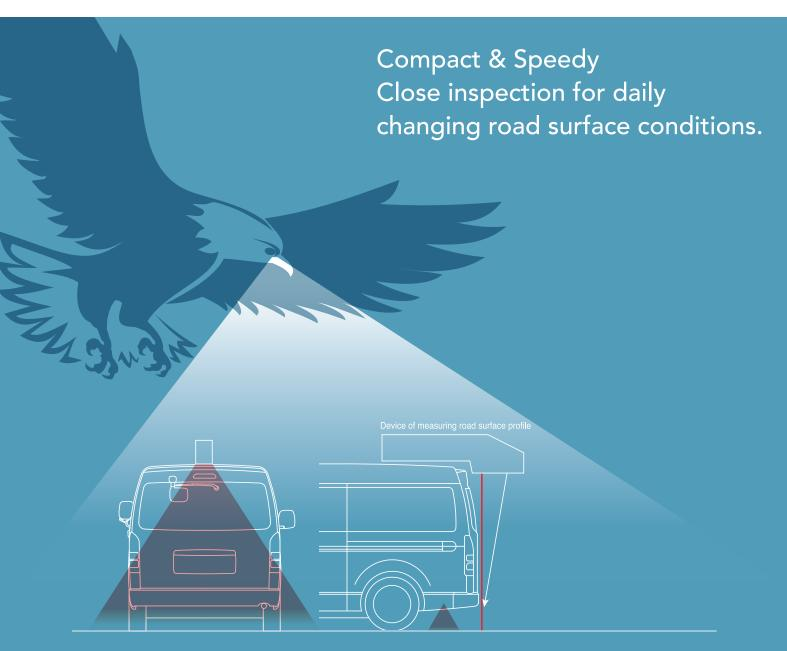
Road surface conditions can be easily inspected by mounting the simple measurement device on a customer's compact car.
